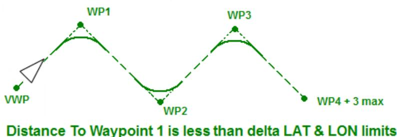
**Step 1.** A regular broadcast event occurs and the own ship has passed the Virtual Waypoint (the ship’s distance to Waypoint 1 is less than LAT & LON  $\pm 209.7151'$ ). There shall be no additional broadcast due to passing the Virtual Waypoint, but any broadcast after passing the waypoint shall use the Virtual Waypoint as the FIRST WP:
