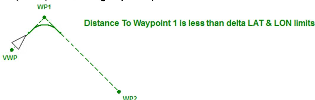
**Step 1.** A regular broadcast event occurs and the own ship has passed the Virtual Waypoint (the ship's distance to Waypoint 1 is less than LAT & LON  $\pm 209.7151'$ ). There shall be no additional broadcast due to passing the Virtual Waypoint, but any broadcast after passing the waypoint shall use the Virtual Waypoint as the FIRST WP:
